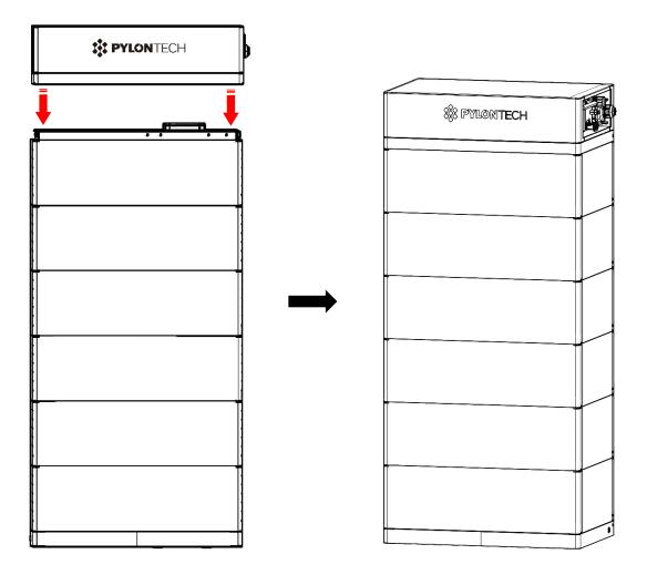
*NOTE*. The above picture is just for reference. The quantity of the battery modules is based on your practical system.
