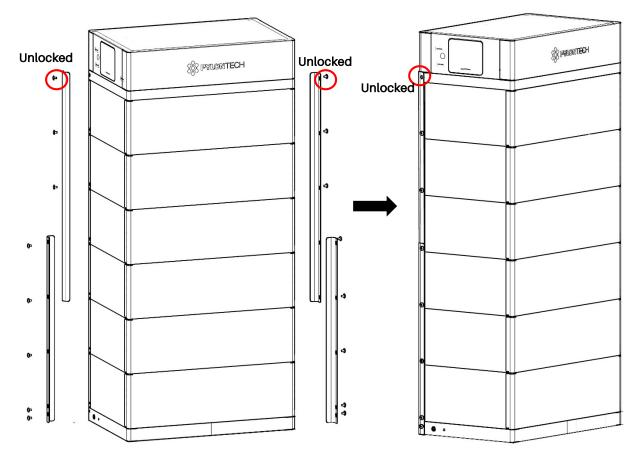
3. Follow the illustrations below, firstly fit the anti-toppling brackets on back sides of the BMS, then use M4 screws to fix.
