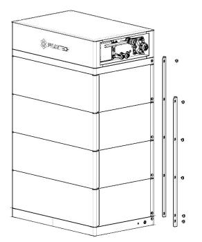
6. Remove the control module and each battery module one by one.
