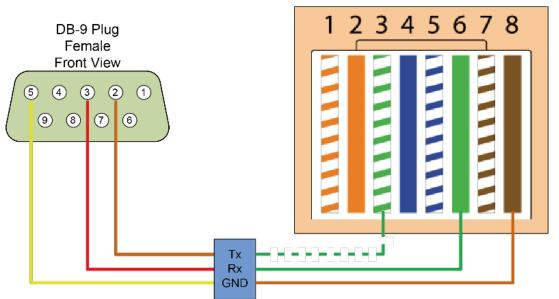
B. If you use a new RS232 debug tool (DB9 – USB), the Pin 8~10 here corresponds to PIN 2,3,5 of DB9 terminal.
