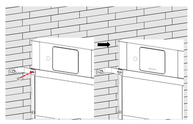
8. Fix the M8 nut (**a**) across the 8mm flat gasket (**c**) and spring washer (**b**), with 12~13N.m torque. Repeat this step for the other bracket.
