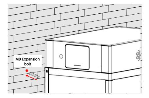
7. Fit the brackets across the M8 expansion bolts on both sides, then fix the brackets on the BMS with M4 screws.
