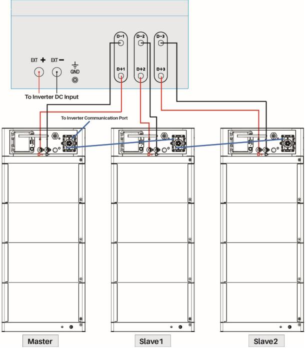
*NOTE*: Make sure to have the D+ & D- plugs into the combiner box properly.
