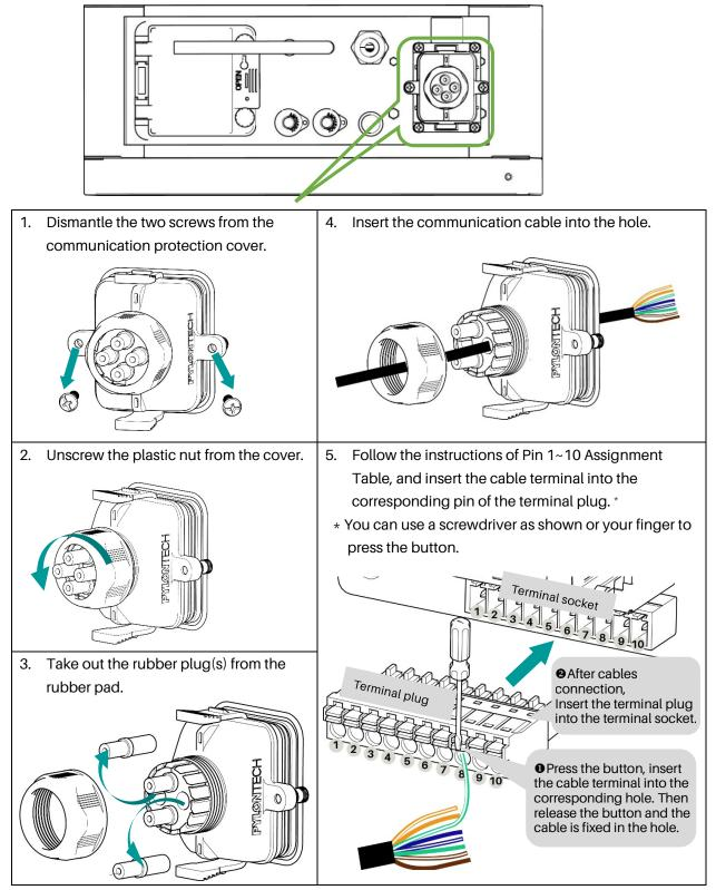
For communication cables connection for PIN1~10 terminal station, please follow the steps below:
