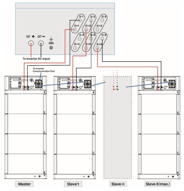
*NOTE*: Make sure to have the D+ & D- plugs into the combiner box properly.
