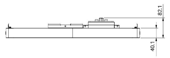
Battery rack basement bitmap (unit: mm)
