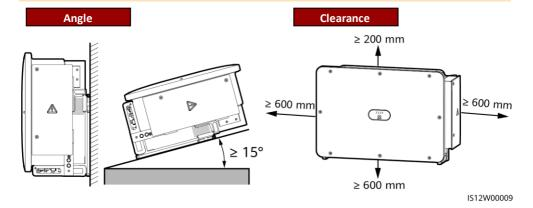
600-730 mm of clearance is recommended underneath.
