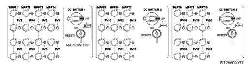
If the number of PV inputs is 11 to 19, the DC input terminals are selected as follows.
