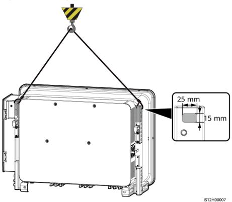
Figure 4-15 Hoisting the solar inverter
