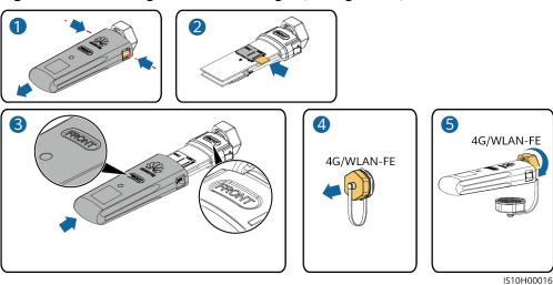
Figure 5-35 Installing a 4G Smart Dongle (SDongleB-06)
