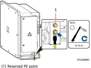
Figure 5-6 Connecting the PE cable to the PE point (on the enclosure)
