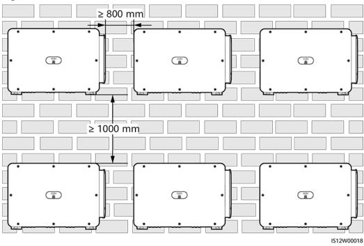
Figure 4-6 Stacked installation mode (not recommended)
