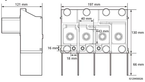
Figure 5-14 AC terminal block dimensions
