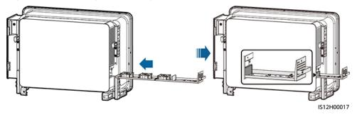
**Step 9** Connect the cables correctly according to the cable labels and bind the cables.
