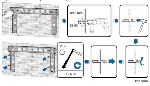
Figure 4-10 Installing the mounting bracket
