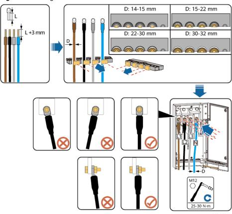
Figure 5-16 Single-core cable connections
