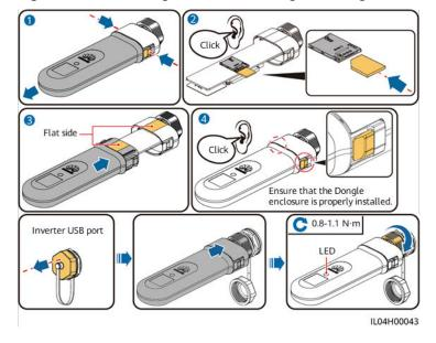
• WLAN-FE Smart Dongle (WLAN Communication)
