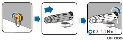
• WLAN-FE Smart Dongle (FE Communication)
