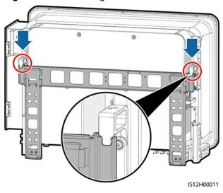
Figure 4-16 Mounting the solar inverter
