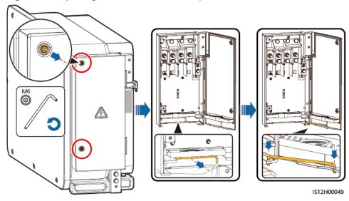
Figure 5-7 Opening the maintenance compartment door
