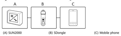
Figure 7-3 Connection over a USB data cable
