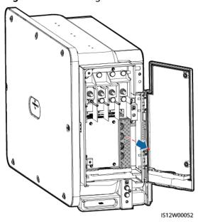
Figure 5-8 Removing the accessories
