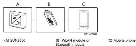
Figure 7-2 Connection over a Smart Dongle
