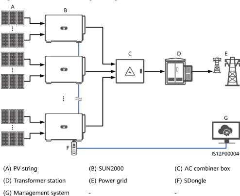
Figure 5-2 RS485 networking (SDongle)
