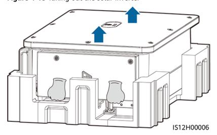
**Step 2** Lift the solar inverter and keep it upright.
