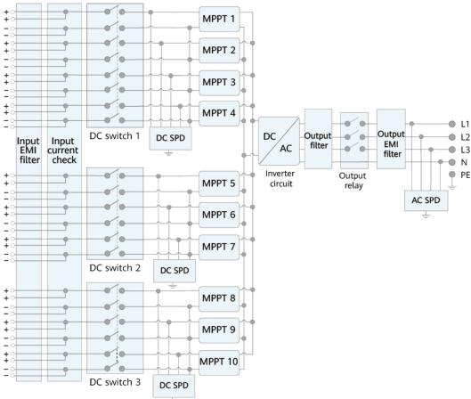
Figure 2-10 Schematic diagram
