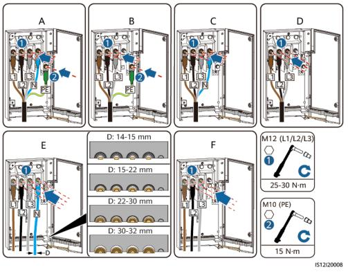
Figure 5-17 Cable connections
